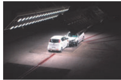
Car to Car 衝突試験設備
